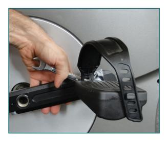
The RAC upgrade kit fits both upright and recumbent exercise bikes that have a 3 piece crank assembly. It simply replaces the existing bike crank with no need to remove the enclosure.
