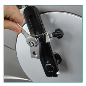
NOTE: The passive arm can also be installed on a standard crank arm.
